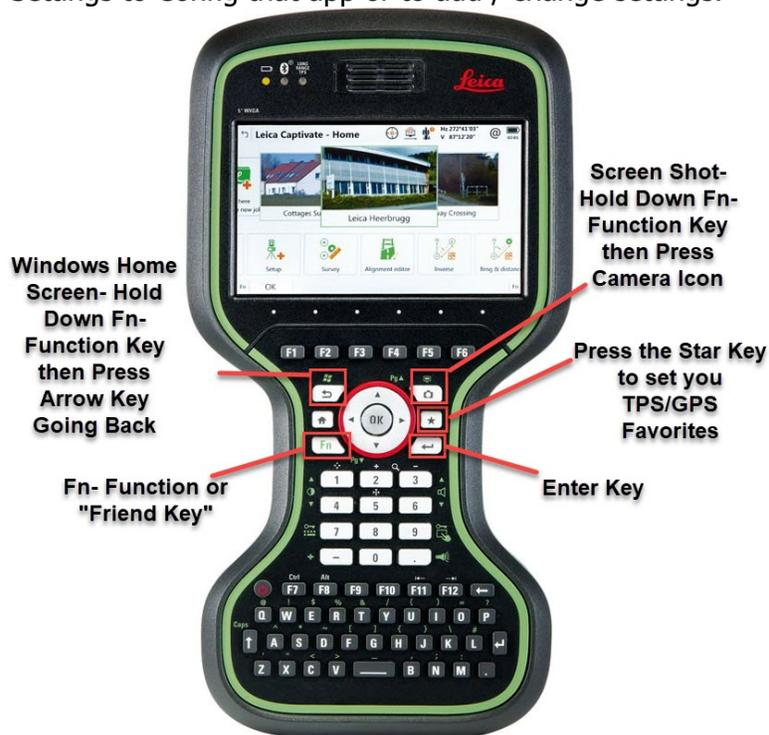
**How to Reset the Windows EC7 within the CS20 Data Collector, remember to not Reset Leica Captivate as this will delete all settings within Leica Captivate even working styles etc.**
