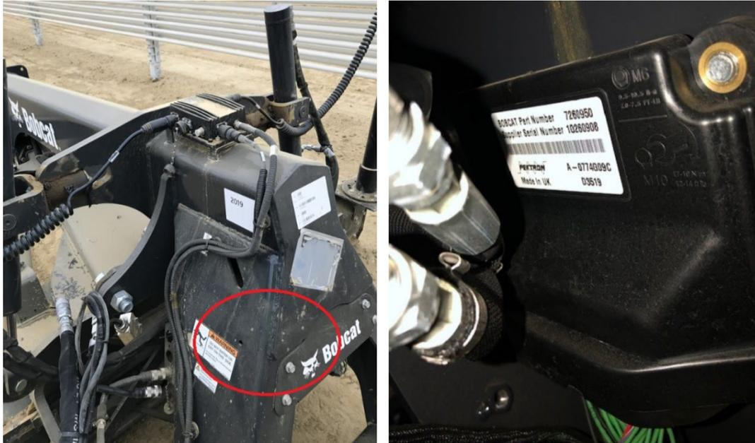
There are several connectors mounted on the sides of the attachment for Trimble sensors, where we can connect our system to the attachment. The connectors contain CAN-Bus and Power pins, so it is possible to get the power connection for the Junction Box
